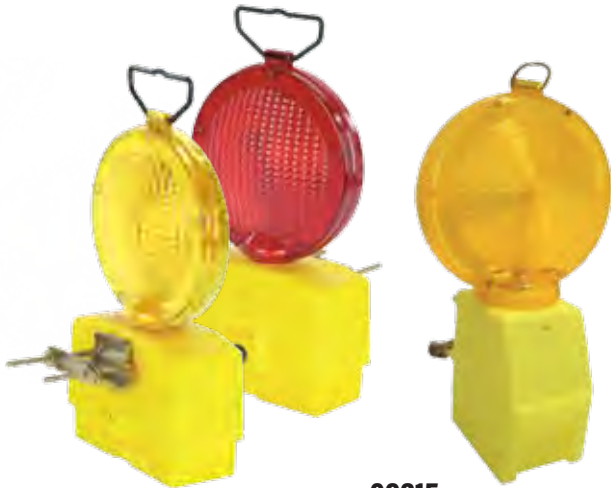
09210 CREPUSCULAR BLINKER Blinker with pole attachment, with fluorescent colour base and crepuscular switch (automatically activates the flashing light when it becomes dark). 2 batteries of 6 volts not included. Colour: Yellow (010) with intermittent light Red (070) with fixed light Full box: 10 pcs.
